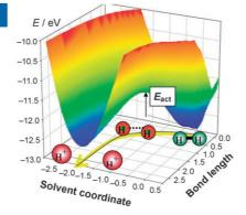
Understanding fuel cell catalysis: The electrochemical oxidation of hydrogen to two protons involves a major reorganization of the solvent. The reaction can be catalyzed by electrodes that have a d band near the Fermi level interacting strongly with hydrogen (see the potential surface for the oxidation of  $H_2$  on platinum).
