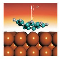
Fivefold versus twofold: Symmetry-breaking interactions in the monolayer of the buckybowl corannulene on Cu(110) lead to the formation of extended mirror domains (see picture). The molecules are adsorbed in a tilted geometry with the bowl opening pointing away from the surface.
